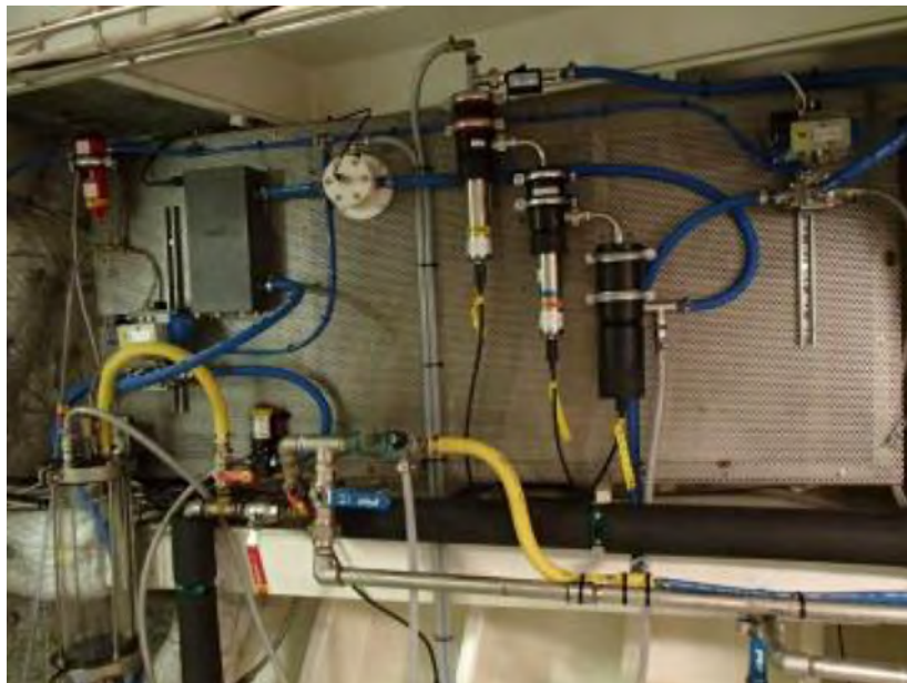
Figure 3.14. Components of a Ferrybox system: Left: sensors for conductivity, oxygen, chlorophyll fluorescence (proxy for phytoplankton biomass), phycocyanin fluorescence (proxy for cyanobacteria biomass), and turbidity Photos: Bengt Karlson; right: an example of a fully configured, commercially available Ferrybox system: http://www.4h-jena.de/ .
