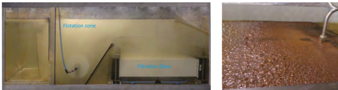
Figure 11.13.7. Side view of the akvoFloat pilot (left) and resulting float layer during operation (right).
