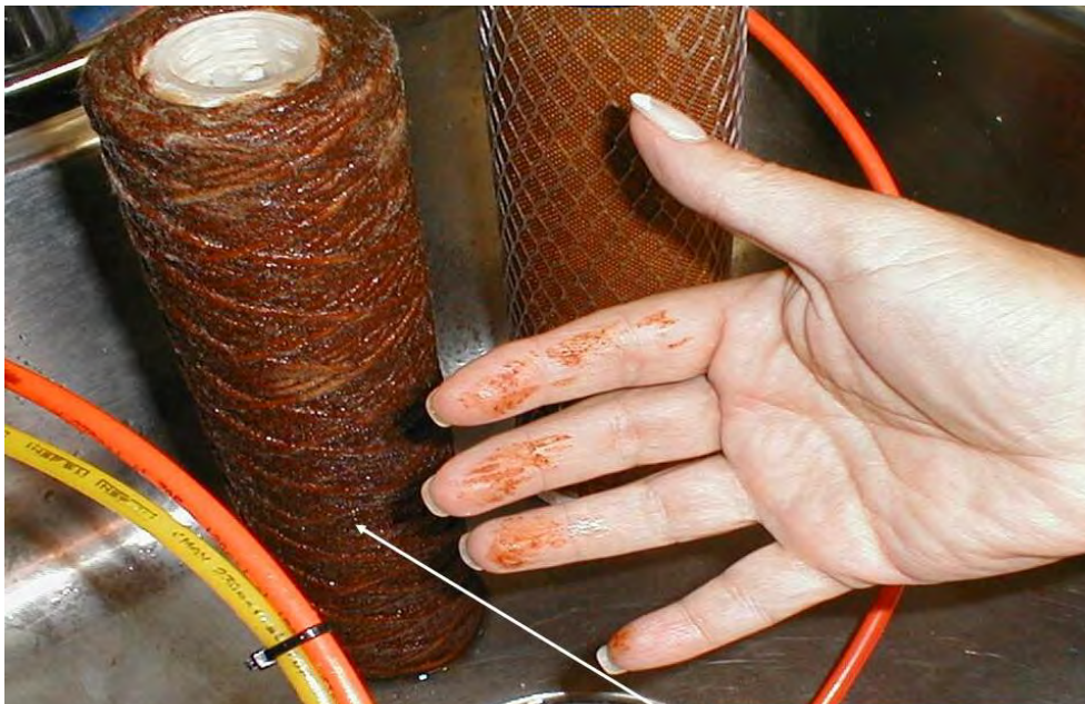
Figure 9.6. Coagulant accumulation on cartridge filters due to overdosing. Photo: Voutchkov 2013.
