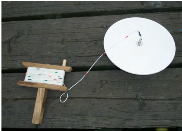
Figure 3.7. A Secchi disc is used to measure water transparency. Photo: B. Karlson.
